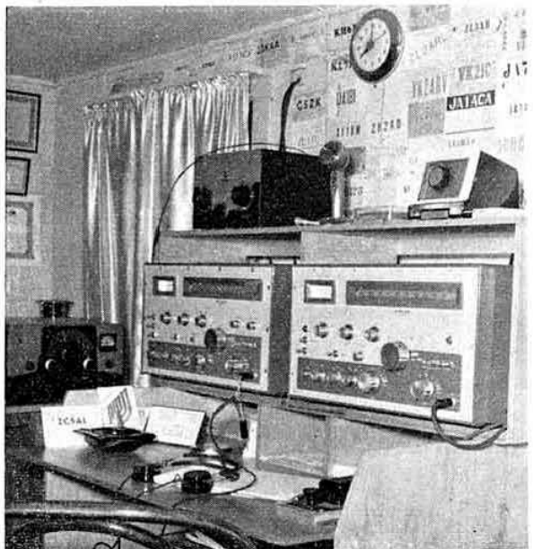
Syd Spencer VE7AMD , of Victoria, British Columbia is the proud owner of this neat station. The transmitter is a Heathkit "Apache" and the receiver a Heathkit "Mohawk." The Johnson "Ranger" transmitter is used as a standby. The aerial is a home-built G3ZU beam. Syd is always happy to work DX stations and adheres to a commendable 100 per cent QSL policy.
